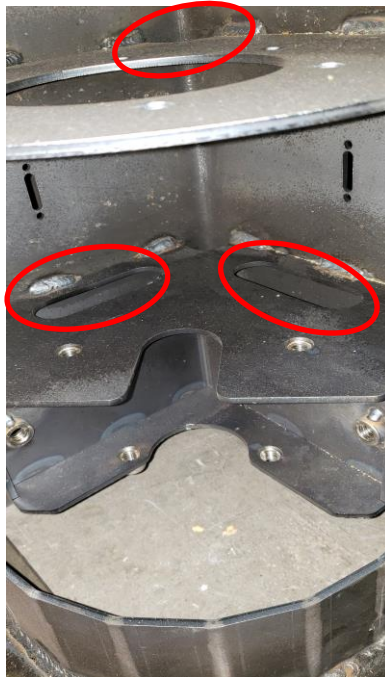
Fig D.4.1 Slot(s) provisions at base plates for wire-runs to the control cabinet
